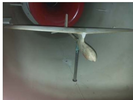
Fig. 6 Wind -Tunnel Model in Yaw Attitude
