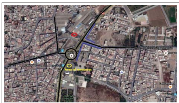
Fig. 10 Location of point sources (red circle), line sources (black lines and circle) and obstacles (blue lines) caused by the buildings surrounding the site (free Google Earth)
