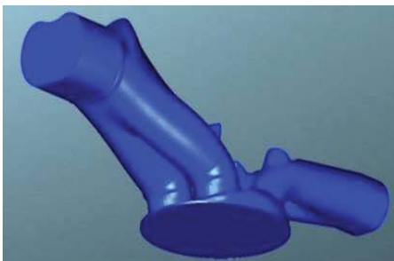
Fig. 2 Perspective view of the chamber geometry layout with 4-valves (bottom view)
