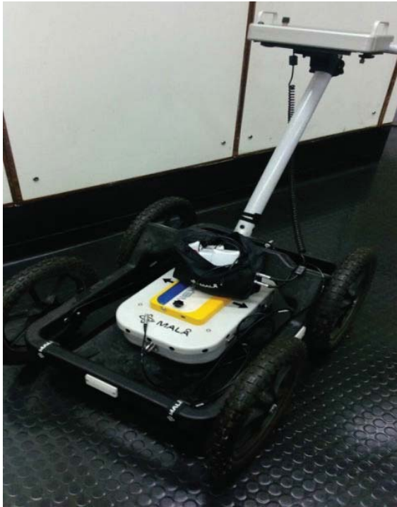
Fig. 1 GPR on a Terraplug Rough Terrain Cart
