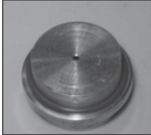
Fig. 7 Photo of the brass injector insert
