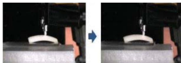
(b) The probe position at the start and end times of the lateral scan
