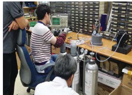
Fig. 4 Performance test of a prototype ammonia detector
