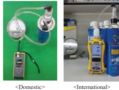
Fig. 4 Comparison Test of combustible gas detectors
