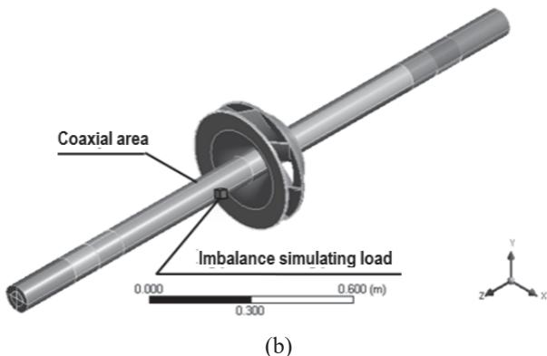
Fig. 8 Modeling of compressor rotor eccentricity: a – in an evident manner; b – by means of a corrective load
