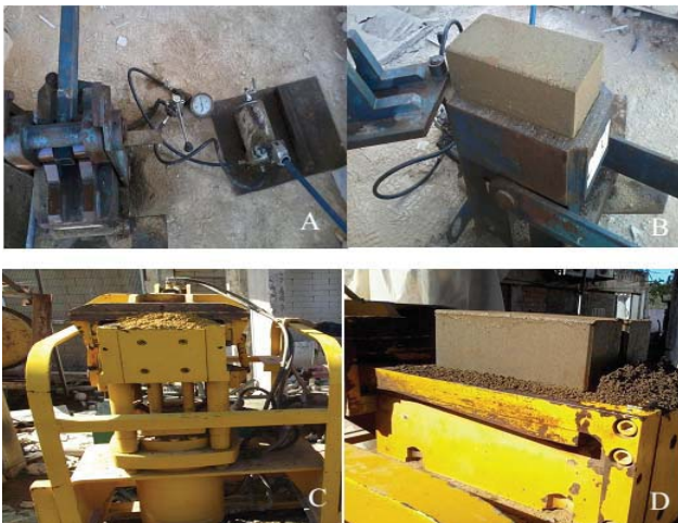
Fig. 2 Compacting types used for samples manufacture
