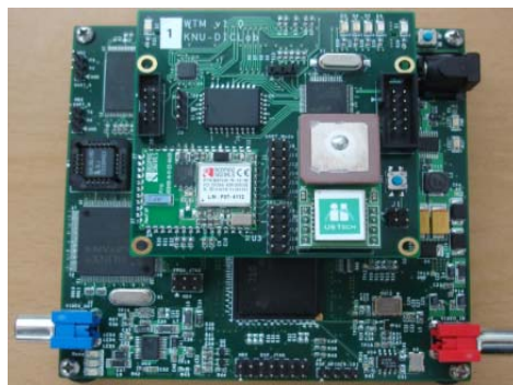
Fig. 8 Picture of implemented H.263 wireless transmitter
