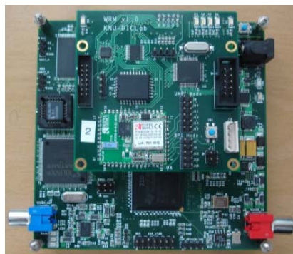
Fig. 10 Picture of implemented H.263 wireless receiver
