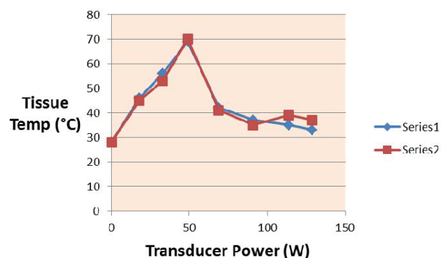
Fig. 6 Cavitation threshold: the relationship between transducer power and tissue heating/cavitation effect
