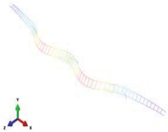
Fig. 4 The Bridge Structure Mode Shape 1
