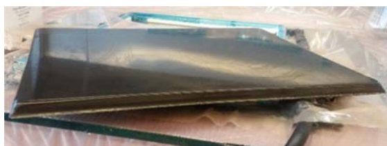
Fig. 2 Core sheets with 3% Boron Nano powder
