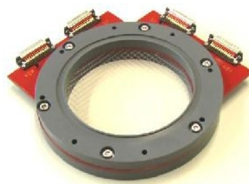
Fig. 1 Design of conductivity wire-mesh sensor
