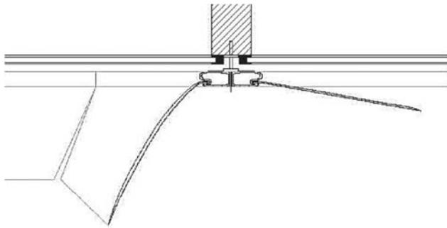
Fig. 9 Detail of flectofin-principle attached to façade-sub construction [11]
