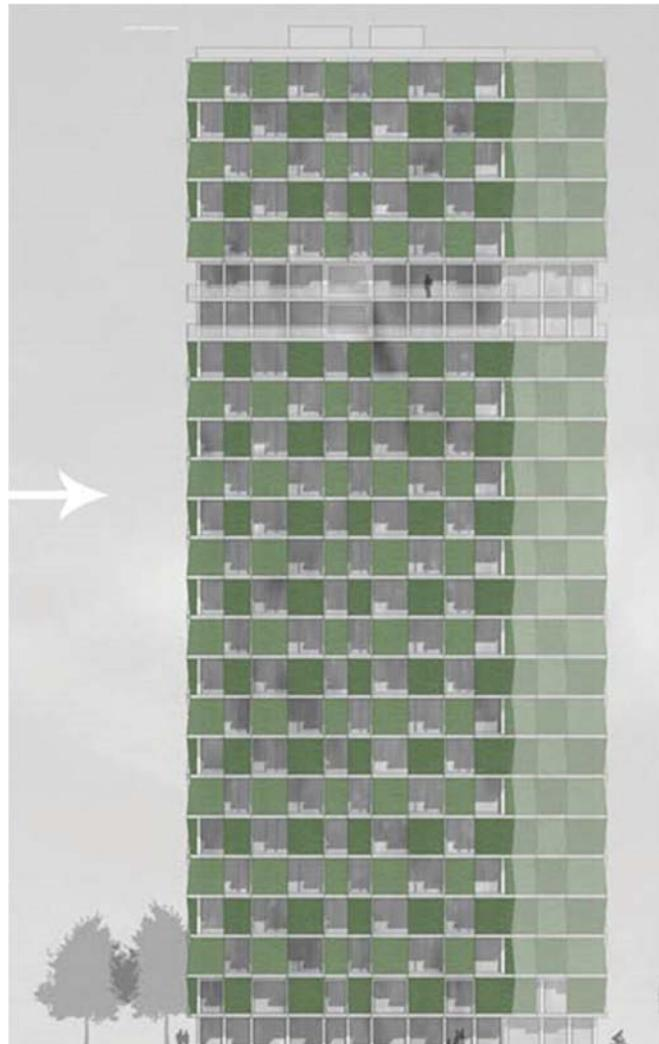
Fig. 5 High-Rise Revisited: Façade -“Müller”-Design using solar ivy [9]
