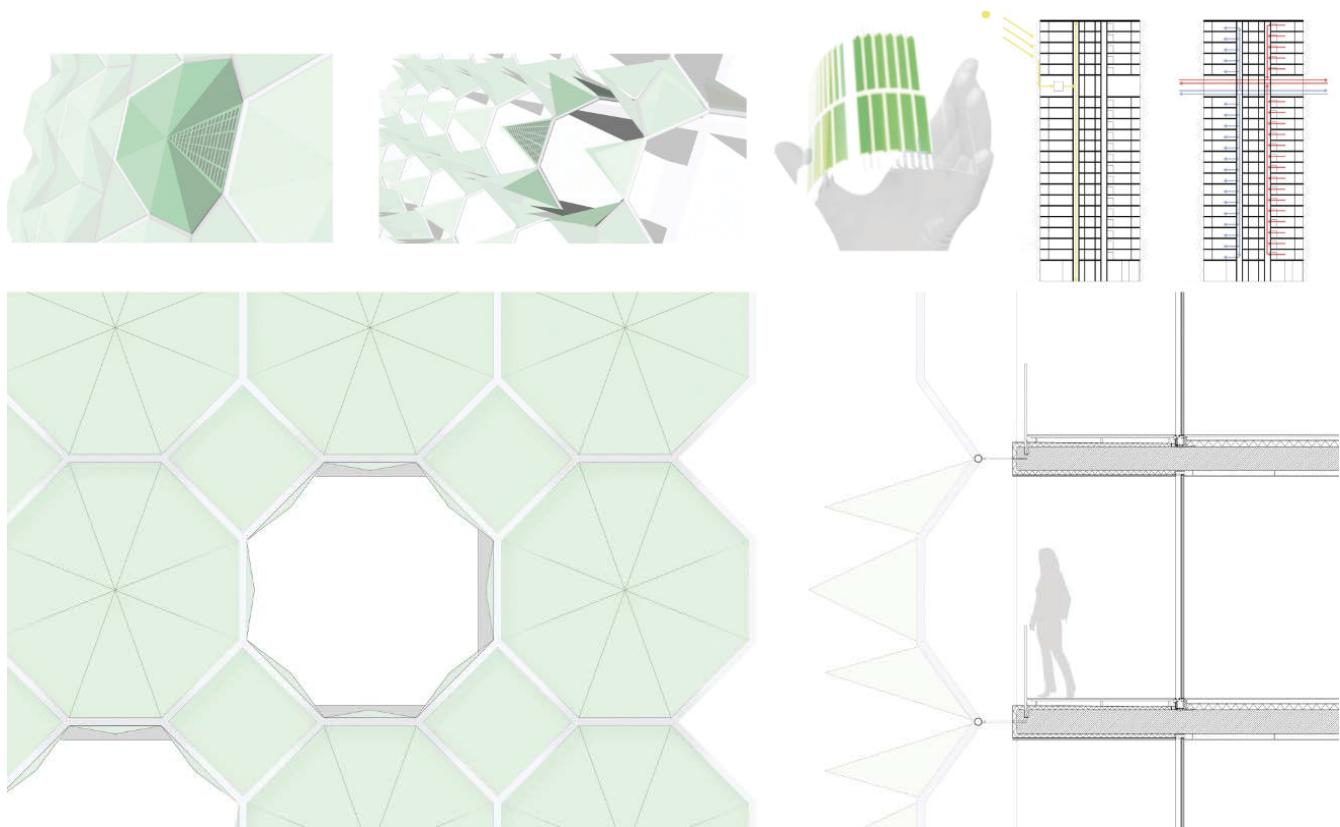
Fig. 15 Octagonal module, each using 8 flectofin-shading-elements [10]
