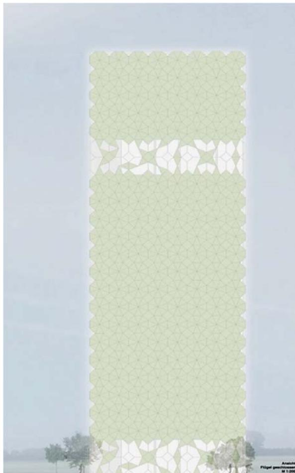
Fig. 16 Façade of “Dittmar”-Design under full solar radiation – elements showing closed state [10]
