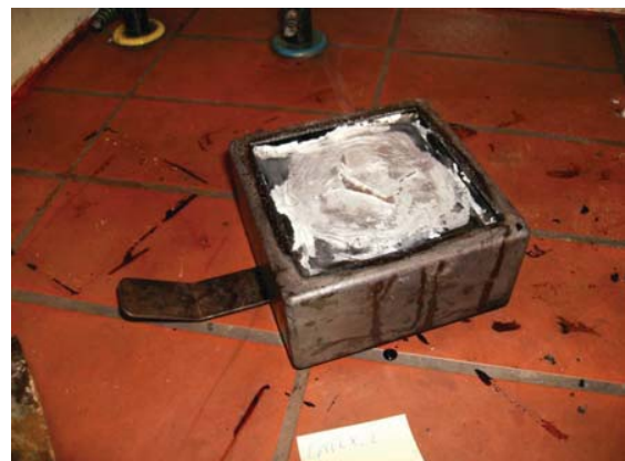
Fig. 14 Detail of the residue to Latex
