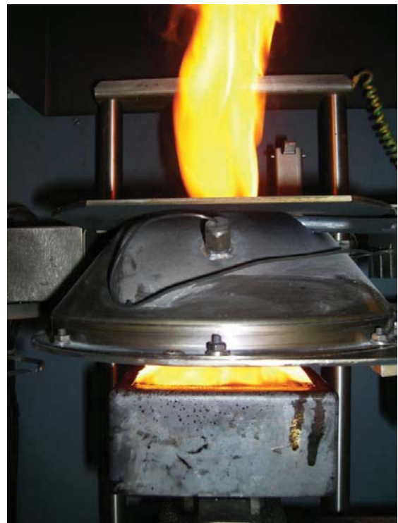
Fig. 13 Burning Latex with detail running and drops through the sample holder
