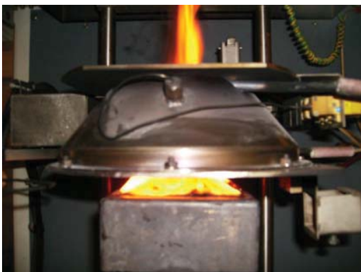
Fig. 7 Detail the behavior of the composites flame 2: 1 and 1:1
