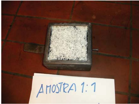
Fig. 10 Detail of the residue of the composite 1:1
