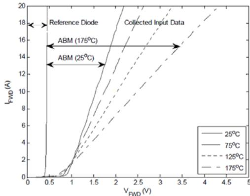
Fig. 2 Voltage drop contributions with current
