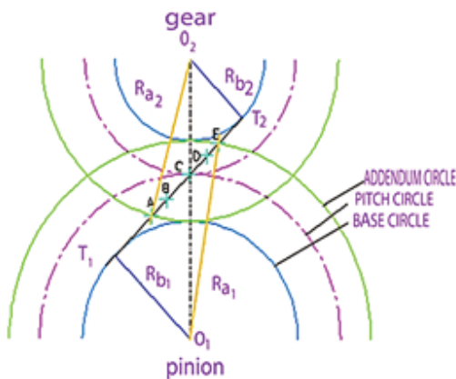
Fig. 1 Path of contact from beginning to end described as A, B, C, D and E (A -Beginning of contact, B1-End of two pair mesh, B2-Beginning of single pair mesh, C -Pitch point, D1-Beginning of two pair mesh, D2-End of single pair mesh, E -End of contact)
