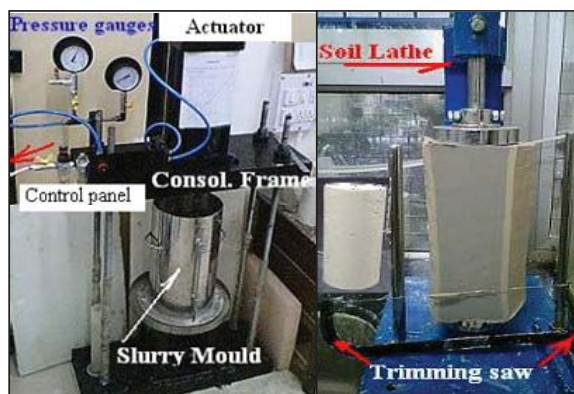
Fig. 2 Consolidation setup on the laboratory floor
