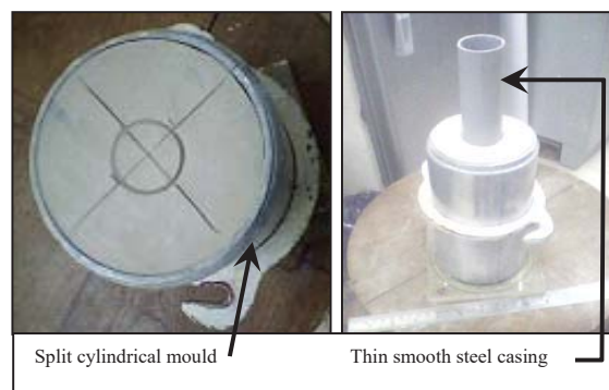
Fig. 3 Preparation of SCP in reconstituted clay specimen
