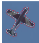
Fig. 4 One example of the adaptation of the initial contour to the edges of the target. Red contour obtained by the neural network, and white contour has been created the greedy snake stage
