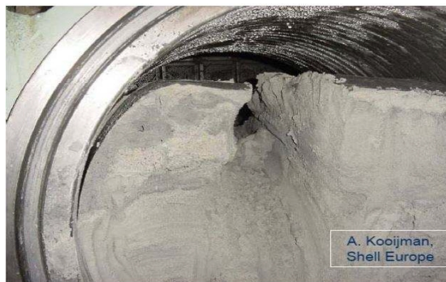
Fig. 2 Sand production at North Sea field [20]
