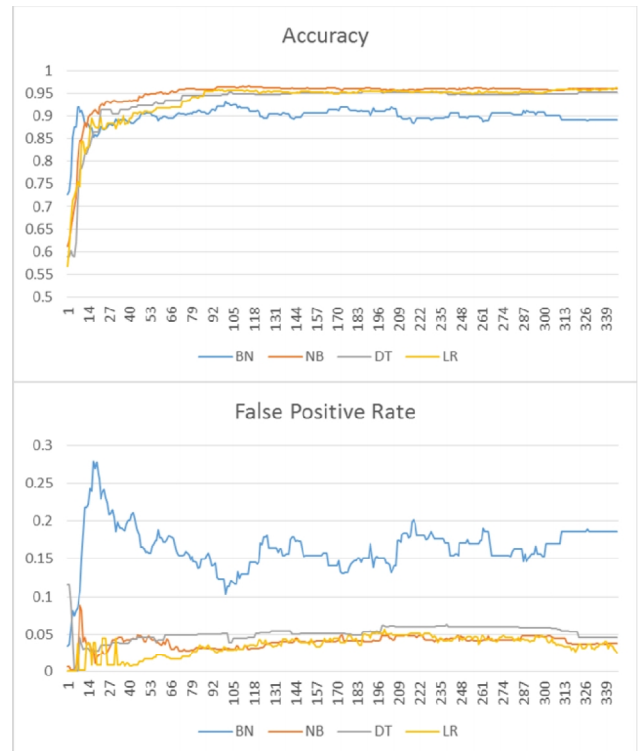
Fig. 7 Learning curves of accuracy and false positive rate for self-applied student who feels inconvenient when the robot vacuum cleaner activated while he works
