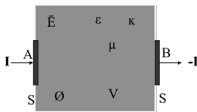
Fig. 1 Electromagnetic model of the tissue exposed to the electric current
