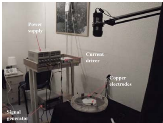
Fig. 3 Experimental setup of Electro-Thermal Imaging System established at Faculty of Medicine, Biophysics Department
