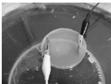
Fig. 5 Homogeneous agar phantom: Current is applied with copper electrodes located at right and left side of the phantom
