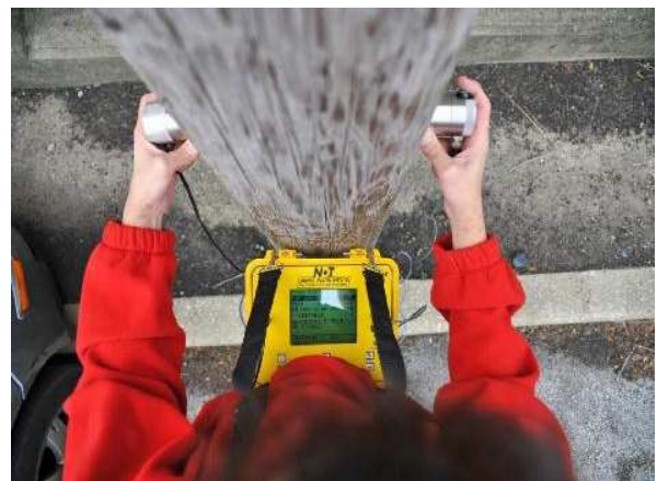
Fig. 6 UPV testing of concrete member
