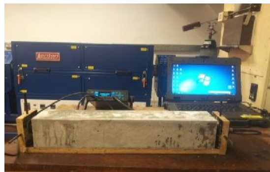
Fig. 1 Ultrasonic pulse velocity test instrument with concrete specimen in position
