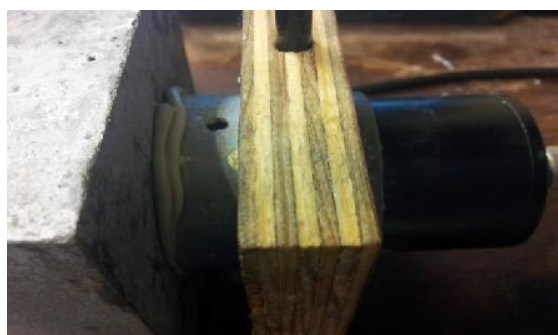
Fig. 3 Testing the concrete specimen with liquid coupling
