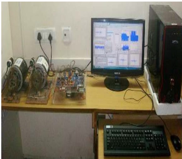
Fig. 3 Experimental setup using healthy and unhealthy motor
