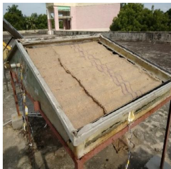
Fig. 2 Jute-Wick arrangement in MDSBMSS setup
