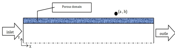
Fig. 2 Schematic of the one homogeneous porous layered structure of an artery wall (not to scale)
