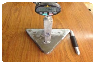
Fig. 8 Mortar bar length reading (compared to metal comparator)
