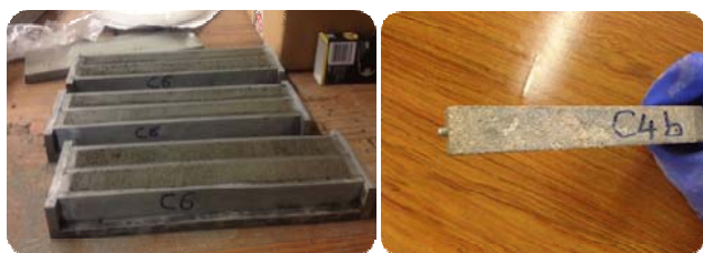
Fig. 6 AMBT molds and mortar bars
