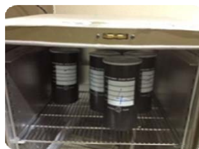
Fig. 7 Storage of mortar bars for AMBT test
