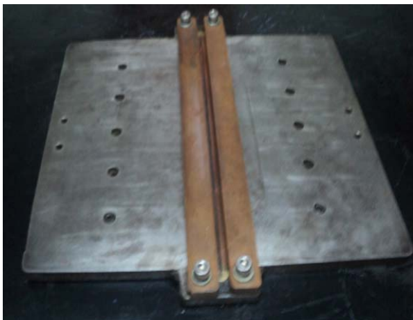
Fig. 6 Work piece clamping system
