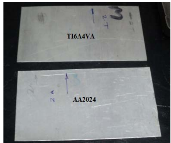
Fig. 4 Ti6Al4V and Aluminium Alloy AA2024
