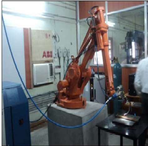
Fig. 5 Nd:YAG laser welding system
