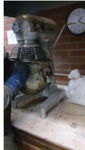
Fig. 3 Aggregate Mixing with Bitumen [7]
