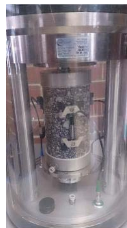
Fig. 11 Final Asphalt Specimen in AMPT [7]
