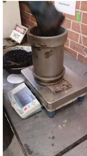
Fig. 4 Molding the Asphalt Sample [7]
