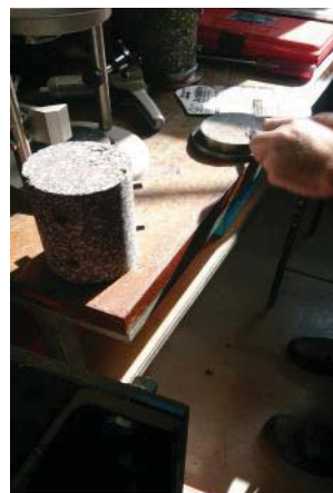
Fig. 9 Final Asphalt Specimen Underwent Gluing Process [7]
