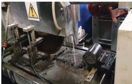
Fig. 7 Asphalt Specimen Undergoing Slab and Core Drill [7]
