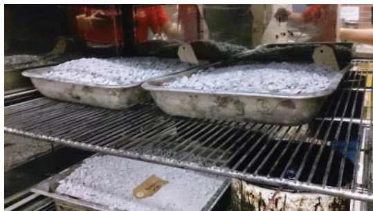
Fig. 2 Final Aggregate Mixture in Asphalt Oven [7]
