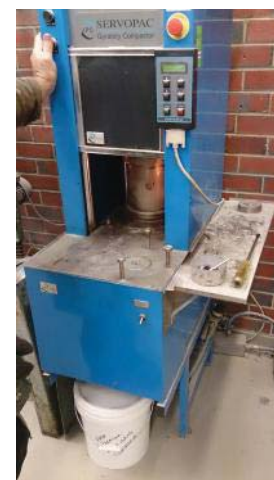
Fig. 5 Gyratory Compaction of Asphalt Specimen [7]
