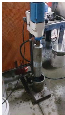
Fig. 6 Asphalt Specimen Undergoing Core Drill [7]
