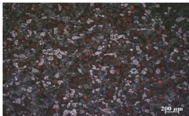
Fig. 6 Photomicrograph of the top side of the Carbon/epoxy PMC Substrate- with the powder layer
