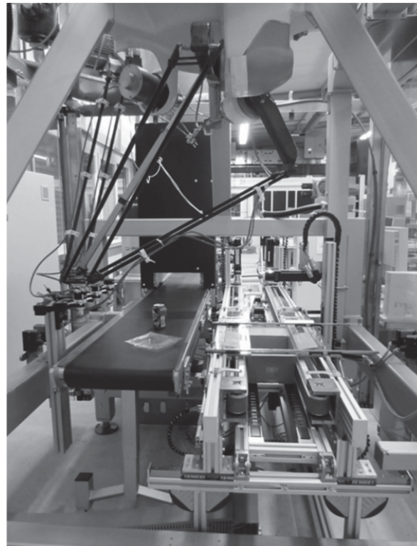
Fig. 15 Demonstrator of a format-flexible case erecting, filling and closing packaging machine
