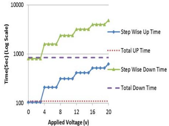
Fig. 8 Step wise and total time consumed for setting of liquid crystal for different increasing and decreasing voltage levels
