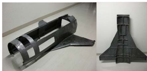
Fig. 14 Full composite semi-monocoque structure of WIRES#014
