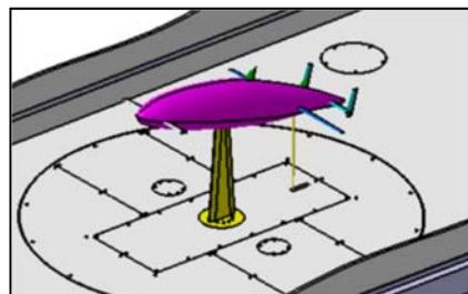
Fig. 4 Isometric view of HB aircraft installed in test section
