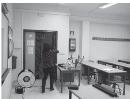
Fig. 2 Airtightness measurement of a classroom
