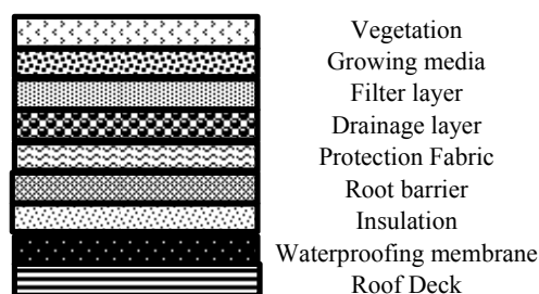
Fig. 1 Structure of green roof system
