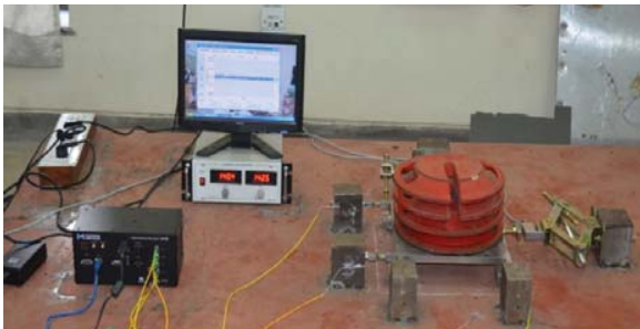
Fig. 3 Experimental setup for calibration of Z axis sensors
