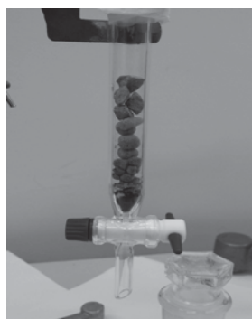
Fig. 1 Column filled with the adsorbents
