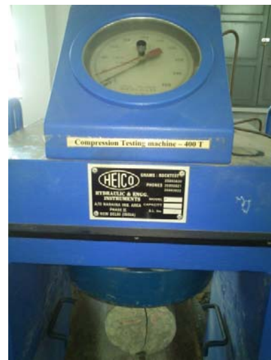
Fig. 10 Split Tensile strength Test
