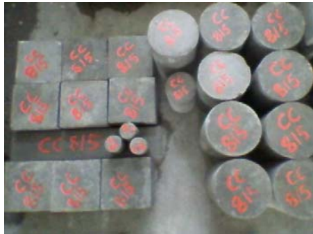
Fig. 5 Casting of Cubes
