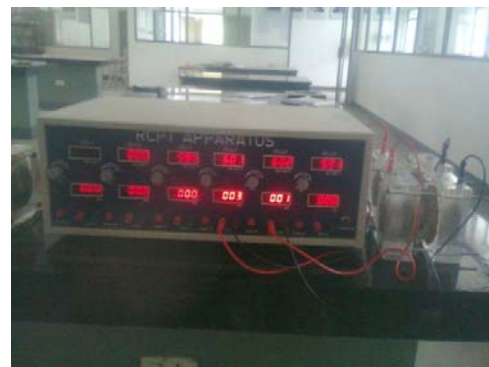
Fig. 16 Rapid chloride Permeability Test
