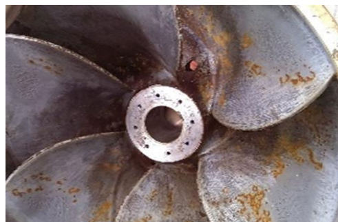
Fig. 16 Cavitation of Impeller
