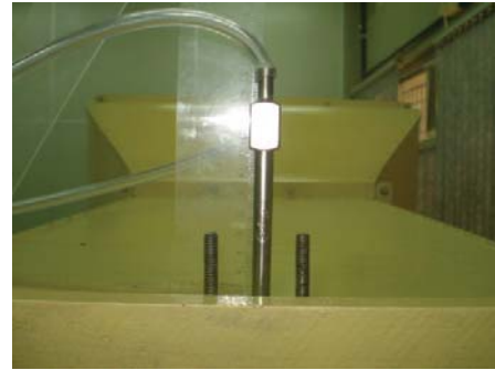
Fig. 4 Height adjustment of the Pitot tube
