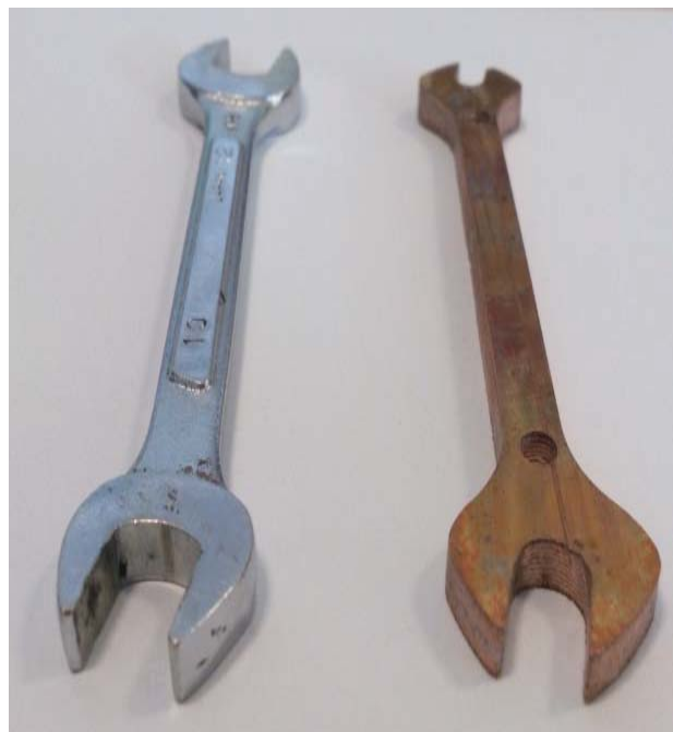
Fig. 13 Composite spanner produced by CMFM
