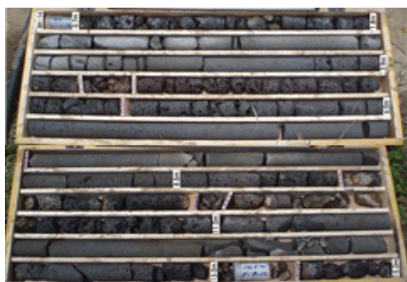
Fig. 2 Core drilling box of polymorphic ground
