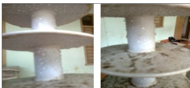
Fig. 4 Appearance of water droplets on the surface of insulator in the early morning hours
