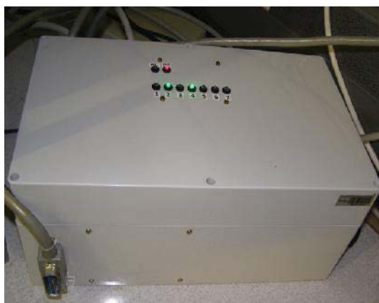
Fig. 4 Programmable GPIB switching isolator (up to 7 channels)
