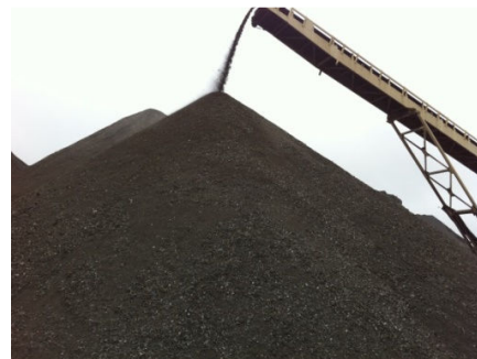
Fig. 1 MSWI bottom ash after treatments
