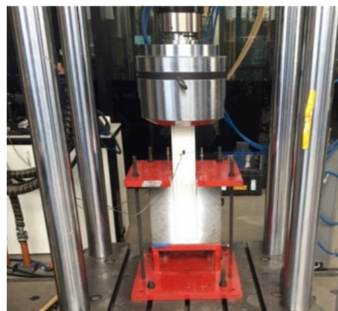
Fig. 1 Control specimen inside the 1MN machine
